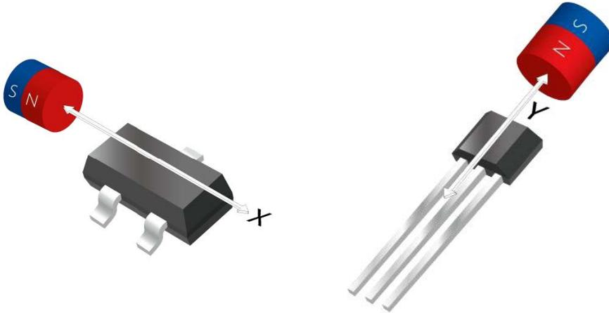
As shown in the Figure 7 below, the KTM1301 can detect magnetic fields parallel to the chip package surface.
