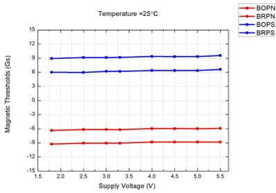
Figure 20: Mag. Thresholds vs. Voltage @ $T_A = 25^\circ\text{C}$
