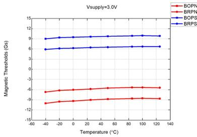
Figure 22: Mag. Thresholds vs.  $T_A$  @ $V_{DD} = 3.0\text{V}$
