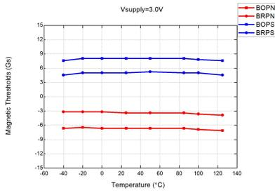
Figure 26: Mag. Thresholds vs.  $T_A$  @ $V_{DD} = 3.0\text{V}$
