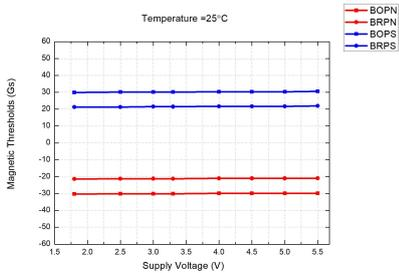
Figure 12: Mag. Thresholds vs. Voltage @  $T_A = 25^\circ\text{C}$
