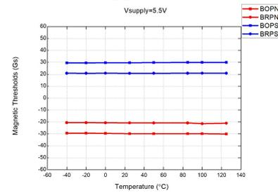
Figure 15: Mag. Thresholds vs.  $T_A$  @  $V_{DD} = 5.5\text{V}$
