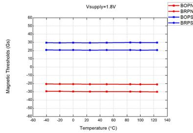
Figure 13: Mag. Thresholds vs.  $T_A$  @  $V_{DD} = 1.8\text{V}$
