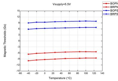
Figure 23: Mag. Thresholds vs.  $T_A$  @ $V_{DD} = 5.5\text{V}$
