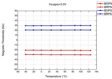
Figure 14: Mag. Thresholds vs.  $T_A$  @  $V_{DD} = 3.0\text{V}$
