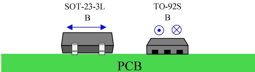
Figure 7: Magnet and Chip Configuration on PCB
