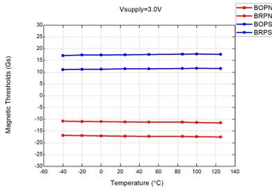
Figure 18: Mag. Thresholds vs.  $T_A$  @ $V_{DD} = 3.0\text{V}$
