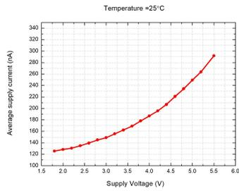
Figure 28: KTM1301SX (50Hz) consu. @ $T_A = 25^\circ\text{C}$
