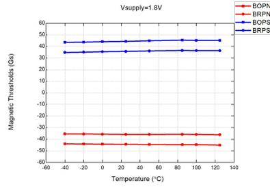
Figure 9: Mag. Thresholds vs.  $T_A$  @  $V_{DD} = 1.8\text{V}$
