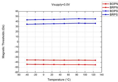
Figure 10: Mag. Thresholds vs.  $T_A$  @  $V_{DD} = 3.0\text{V}$
