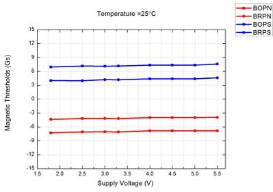
Figure 24: Mag. Thresholds vs. Voltage @ $T_A = 25^\circ\text{C}$
