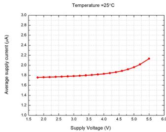
Figure 30: KTM1301TX (continuous operation) consu. @ $T_A = 25^\circ\text{C}$
