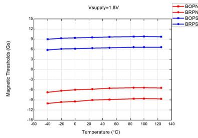
Figure 21: Mag. Thresholds vs.  $T_A$  @ $V_{DD} = 1.8\text{V}$
