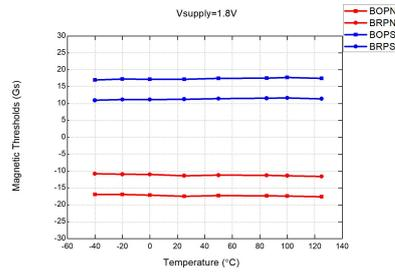
Figure 17: Mag. Thresholds vs.  $T_A$  @ $V_{DD} = 1.8\text{V}$
