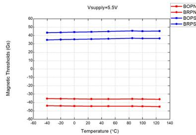
Figure 11: Mag. Thresholds vs.  $T_A$  @  $V_{DD} = 5.5\text{V}$
