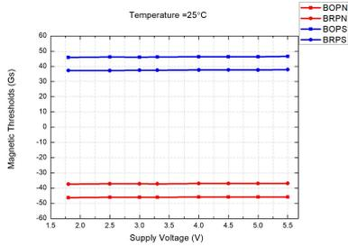
Figure 8: Mag. Thresholds vs. Voltage @  $T_A = 25^\circ\text{C}$
