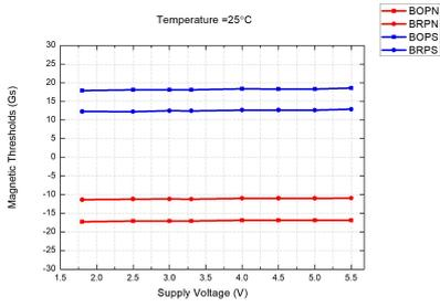
Figure 16: Mag. Thresholds vs. Voltage @ $T_A = 25^\circ\text{C}$
