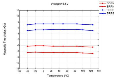
Figure 27: Mag. Thresholds vs.  $T_A$  @ $V_{DD} = 5.5\text{V}$
