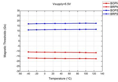
Figure 19: Mag. Thresholds vs.  $T_A$  @ $V_{DD} = 5.5\text{V}$
