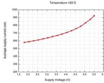
Figure 29: KTM1301MX (1.6kHz) consu. @ $T_A = 25^\circ\text{C}$
