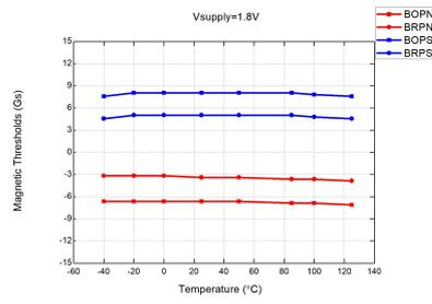
Figure 25: Mag. Thresholds vs.  $T_A$  @ $V_{DD} = 1.8\text{V}$
